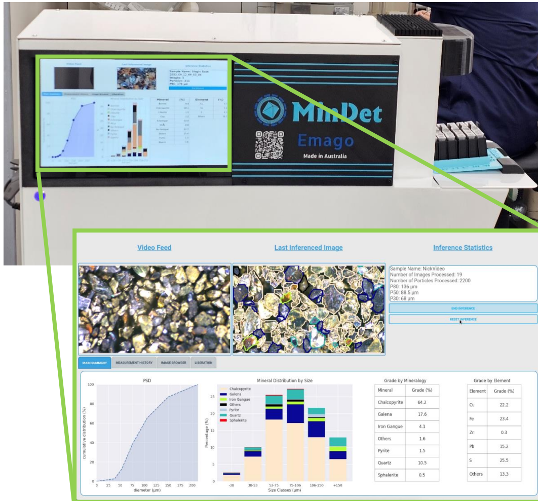
Figure 2 – Emago, the laboratory mineral identification device and the MinDet software User Interface (UI).
