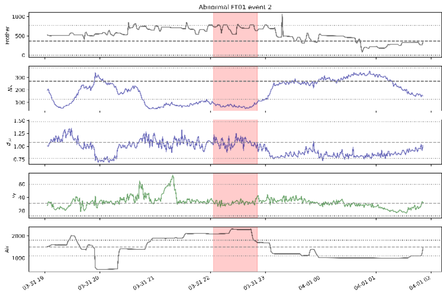
Figure 12: FT01 abnormal event #2 responses (highlighted in red) with preceding and subsequent time series included.
